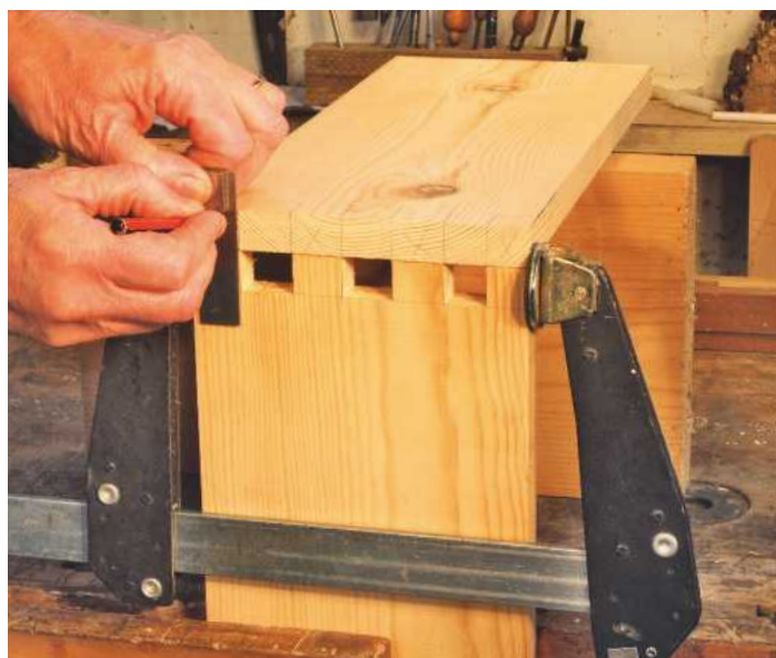
▲ Pic.12 Method of transferring marks for the fingers as a practice for dovetails
